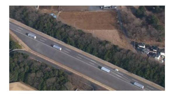
(Phys.org) —Japan's New Energy and Industrial Technology Development Organization (NEDO) has tested a caravan of self driving trucks. They put four trucks on the road, with the first truck driven by a human, followed by three autonomous trucks. The caravan successfully used technologies for steering, for maintaining speed, and for staying in formation, at a speed of 80km/h with a four-meter distance between each truck.
