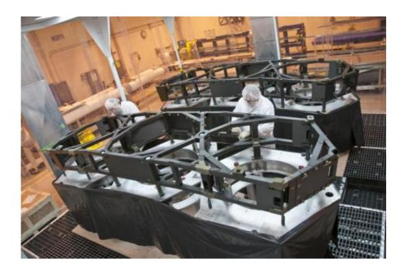
Technicians complete the primary mirror backplane support structure wing assemblies for NASA's James Webb Space Telescope at ATK's Space Components facility in Magna, Utah. ATK recently completed the fabrication of the primary mirror backplane support structure wing assemblies for prime contractor Northrop Grumman on the Webb telescope. Credit: Credit: Northrop Grumman/ATK
