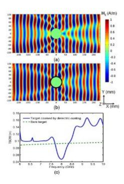
a) shadow behind metal cylinder under plane wave illumination; b) front reconstruction after passing cylinder cloaked by thin multilayer dielectric; c) total scattering cross width for cloaked & bare cylinders. (b) & (c) demonstrate the cloaking effect.
