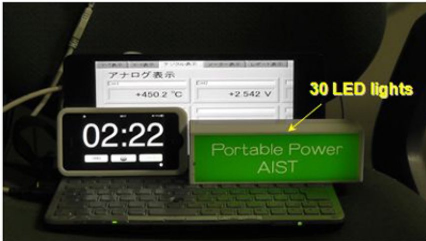
Figure 4: Driving test of USB device (LED light) using LPG cartridge fuel. In principle, 24-hour continuous operation per cartridge is possible.
