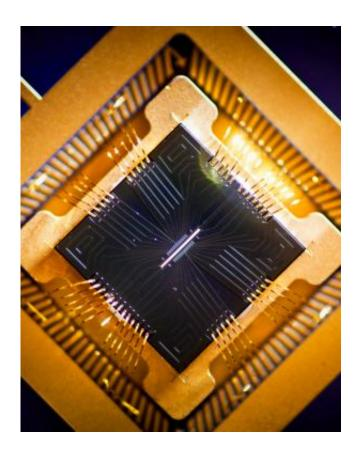
Surface trap fabricated by Sandia National Labs, supported by IARPA. This type of trap has been used to capture ions at JQI and Duke University, as well as other institutions. The image shown here appears on the cover of this week's issue of *Science* magazine. Credit: JQI
