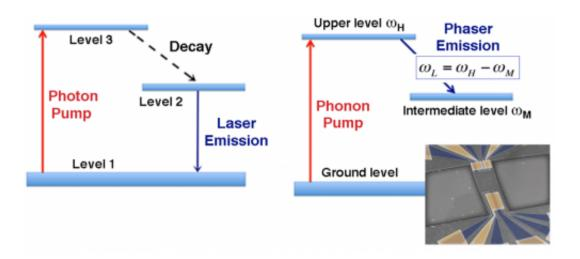
(Left) Three-level scheme for a conventional optical laser. (Right) Three-level scheme of the phonon laser reported by Mahboob et al. Credit: APS/José Tito Mendonça; Image on homepage and inset: I. Mahboob/NTT Basic Research Laboratories
