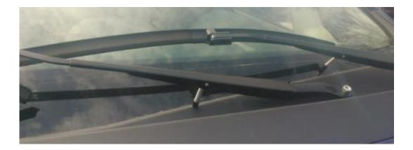
Pegs lift wiper blades to keep them from freezing to car windshield. Below, a close-up.
