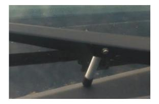
The peg doesn't affect the operation of the wipers at all. Exiting the car, the driver manually flips them down against the windshield when snow or ice is forecast, but just a flip of the car's wiper switch resets the wiper blades to their intended position against the windshield.
