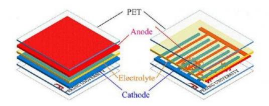
(Left) In the sandwich structure, the two electrodes occupy different layers and face each other. (Right) In the new comb-teeth structure, the two electrodes are integrated in the same plane. The empty space in between them allows for the structure to be flexible and semitransparent. Credit: Heng Lit, et al. ©2013 American Chemical Society
