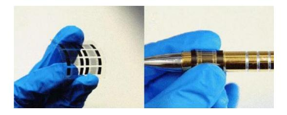
Solar cells made with the electrode comb-teeth structure show good semitransparency and flexibility, as demonstrated by being wrapped around a 9-mm-diameter pen. Credit: Heng Lit, et al. ©2013 American Chemical Society
