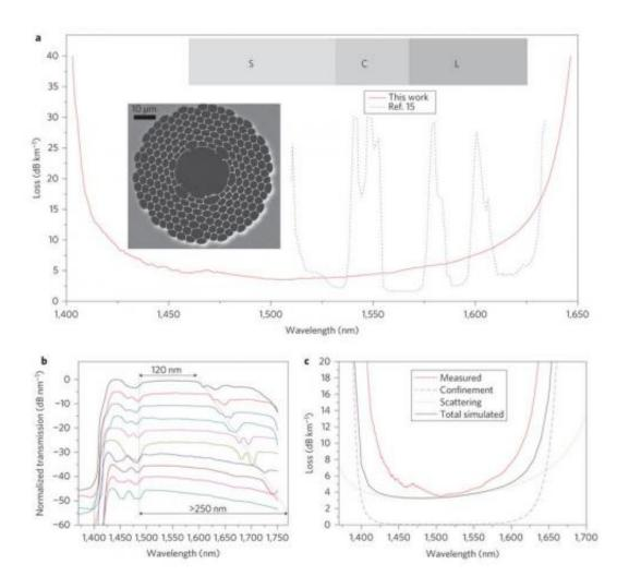
Fabrication and characterization of wide-bandwidth HC-PBGF. Credit: *Nature Photonics* (2013) doi:10.1038/nphoton.2013.45
