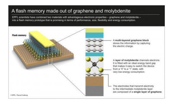
EPFL scientists have combined two materials with advantageous electronic properties -- graphene and molybdenite -- into a flash memory prototype that is promising in terms of performance, size, flexibility and energy consumption. Credit: EPFL
