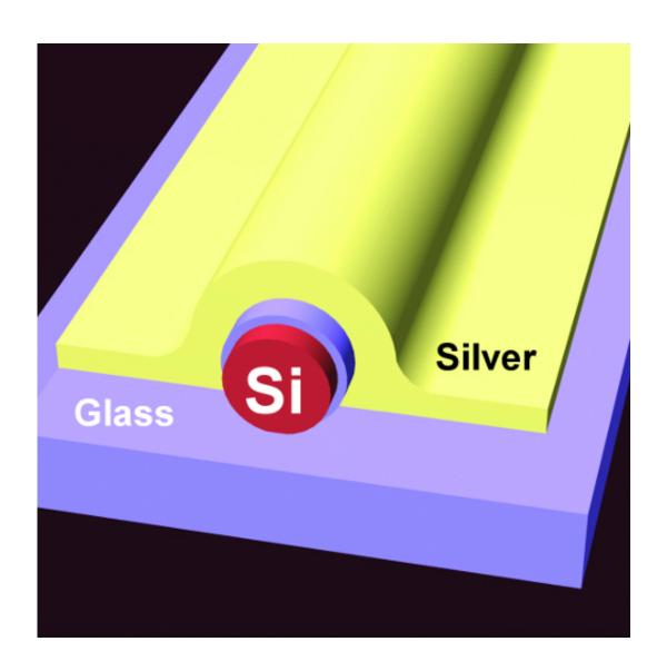
This is a schematic of silicon nanowire integrated with an omega-shaped metal nanocavity. Credit: University of Pennsylvania
