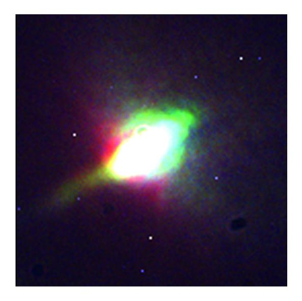
This shows white light emission from silicon coupled with nanocavity under laser excitation. Credit: University of Pennsylvania
