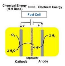
Burning hydrogen in a fuel cell generates an electrical current. A new iron-based catalyst might help make those fuel cells less expensive.
