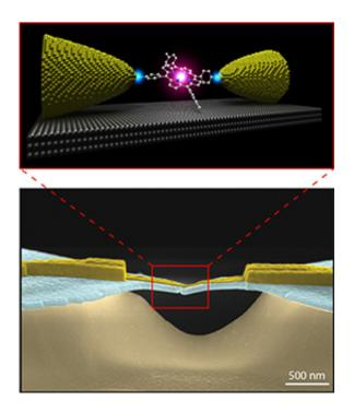
Diagram (top) of a molecule that has been attached to two gold electrodes (yellow in the figure). Electron microscopy image (below) of a break junction. The golden metal strip is broken in the middle; in the opening created a molecule is placed on which measurements can be performed.
