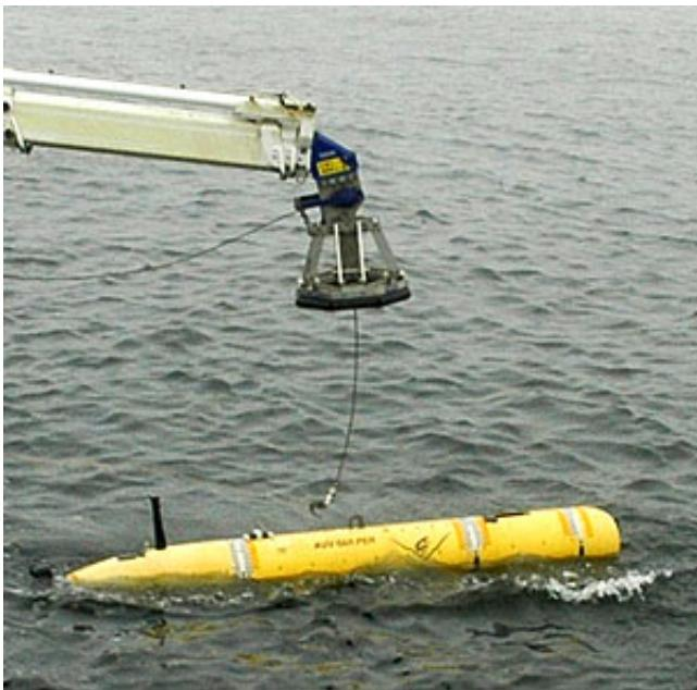
This photo shows MBARI's "Gulper" AUV being launched from the research vessel Rachel Carson. Credit: John Ryan
