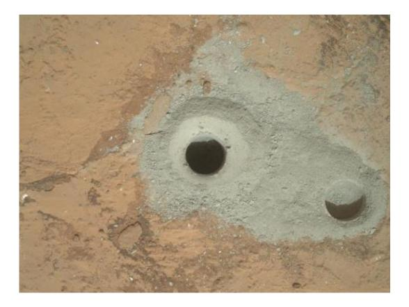
Curiosity's First Sample Drilling hole is shown at the center of this image in a rock called "John Klein" on Feb. 8, 2013, or Sol 182 operations. The image was obtained by Curiosity's Mars Hand Lens Imager (MAHLI). The sample-collection hole is 0.63 inch (1.6 centimeters) in diameter and 2.5 inches (6.4 centimeters) deep. The "mini drill" test hole near it is the same diameter, with a depth of 0.8 inch (2 centimeters). Credit: NASA/JPL-Caltech/MSSS
