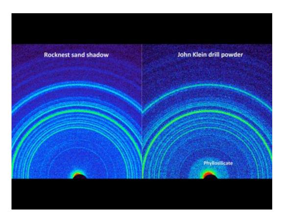
This side-by-side comparison shows the X-ray diffraction patterns of two different samples collected from the Martian surface by NASA's Curiosity rover. Image credit: NASA/JPL-Caltech/Ames
