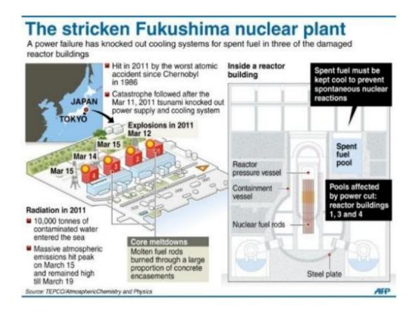
Graphic showing the stricken Fukushima nuclear plant in Japan where a power cut has forced the operator to shut down the cooling system for spent fuel pools.
