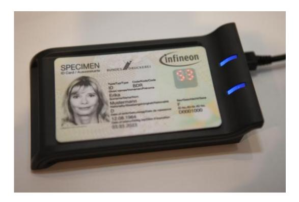
The new security smart card developed by Infineon Technologies and Bundesdruckerei boosts the security of authentication and payment applications: in addition to the static password, a dynamic PIN is requested and automatically generated for each transaction by the security chip in the card and displayed on the integrated LED display.
