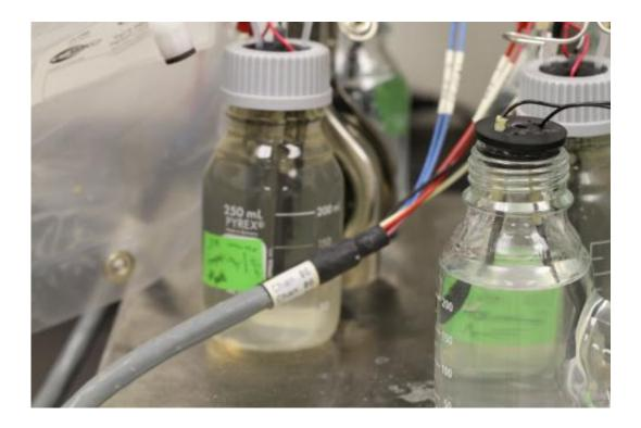
Bench-top Microbial Fuel Cell (MFC): Bacteria attach themselves to the anode of a battery and transfer their electrons to the metal. These electrons then flow to the cathode side, generating useable electricity in the process. An alternate form of the device produces hydrogen at the cathode. Credit: The Biodesign Institute at Arizona State University
