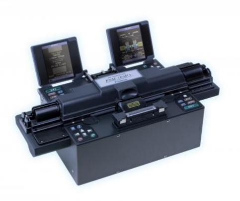
The Fujikura FSM-100P+ fusion splicer is used for the automated alignment and splicing of MCF with PC control software developed by AFL. Credit: Image courtesy Fujikura Splicer Department
