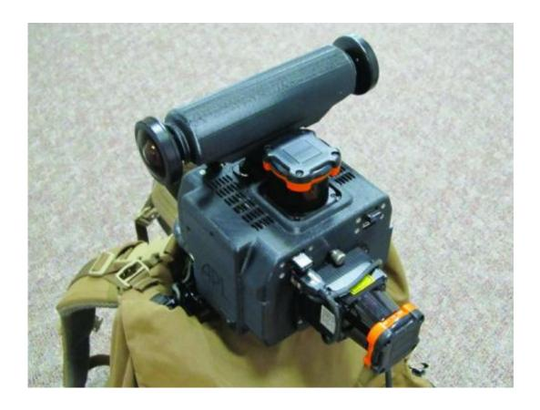
This is a closeup of the backpack-carried Enhanced Mapping and Positioning System, or EMAPS. Credit: Johns Hopkins University Applied Physics Laboratory
