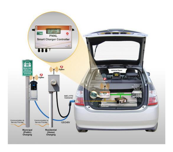
AeroVironment, Inc. has licensed a technology from PNNL that will allow widespread adoption of plug-in electric vehicles without negatively impacting the electrical grid. The PNNL technology tells a vehicle's battery charger when to start and stop charging based upon existing conditions on the electrical grid. AeroVironment will use a portion of the licensed technology in a new prototype version of its Level II charging systems.
