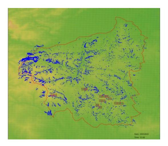
An example of one of the risk maps for Burgenland in Austria. The red boxes mark areas with an elevated risk of landslides. Credit: Fraunhofer IOSB
