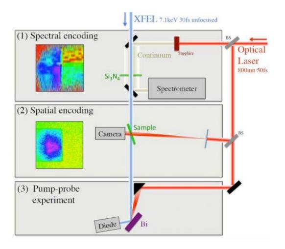
This diagram shows the path of X-ray pulses (blue) and pulses from a separate laser (red) and a sequence of measurement tools that provide a highly accurate gauge of the arrival times of each laser. Credit: Nature Photonics
