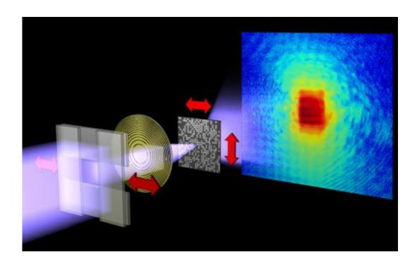
While the test object is moved through the X-ray beam with nanometer precision, the scattered X-rays are captured by a detector. The scattering images are then reconstructed to an image of the sample. Credit: Technische Universitaet Muenchen / Paul Scherrer Institute, Villigen (Switzerland)
