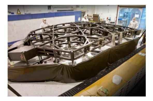
Engineers at ATK work on the center section of the "backplane" support structure that will hold Webb's mirror segments. Credit: ATK
