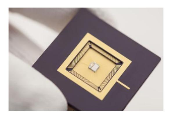
At this week's International Solid State Circuits Conference (ISSCC 2013), imec and Holst Centre presented an ultra-low power processor that operates reliably at near-threshold voltages. The processor delivers clock speeds up to 1MHz at voltages down to 0.4 V. In tests based on a Fast Fourier Transform use case, it consumed only 79  $\mu$ W – a fraction of the power consumption at standard voltages.
