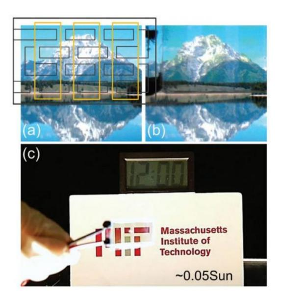
2(a) Picture of the "Teton mountains" displayed on an LCD screen 2(b) with the fully assembled transparent solar cell in front of the picture. In 2(a) the anode/active layer drawing is overlaid on the same picture and the orange boxes
