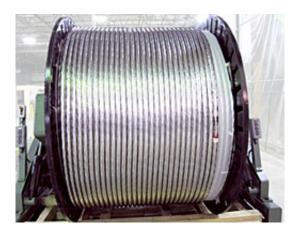
Superconducting strand is cabled at New England Wire Technologies on 2.5 meter wide by 2 meter tall spools before shipment to Florida for conductor jacketing. Credit: NEWT
