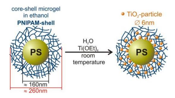
The nanoparticles crystallize in a polymer network at room temperature. Credit: HZB
