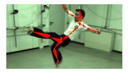
Actors in their normal clothing are filmed with ordinary cameras. The movements are then analysed with special computer software and transferred to a virtual character in the form of a skeleton. Credit: MPI for Informatics
