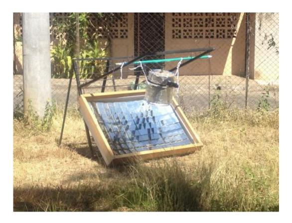
The SolarClave system in operation. It takes up to an hour to heat up to sterilizing temperature, then about 20 minutes to complete the sterilizing cycle. PHOTO COURTESY OF ANNA YOUNG AND JOSÉ GÓMEZ-MÁRQUEZ
