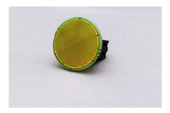
The plate for performing electroporation has the shape of a disk and it is a little smaller than a 20 cent coin. Credit: UPC
