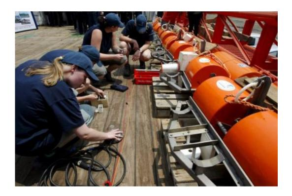
German crew members install ocean bottom Seismometers which formed part of a tsunami early warning system in the Indian ocean. Credit: AAP/Mast Irham
