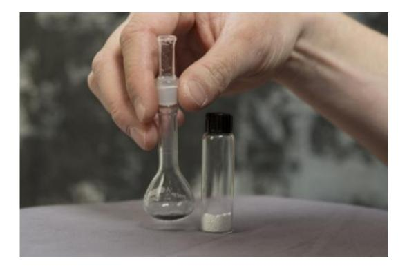
UD researcher Erik Koepf with two vials -- that on the left contains solar fuel and that on the right contains zinc oxide powder, which is placed into the reactor and exposed to high concentrations of sunlight to produce the solar fuel.
