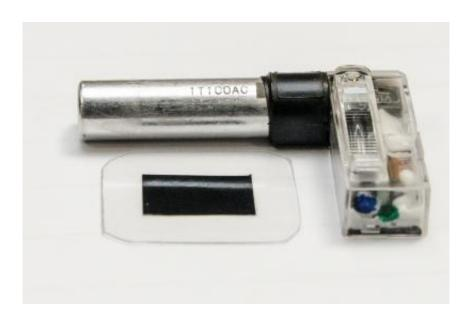
This shows a mobile phone flash unit with its existing capacitor (silver cylinder) compared with NTU's new super thin polymer capacitor material (which is the black colour material). Credit: Nanyang Technological University
