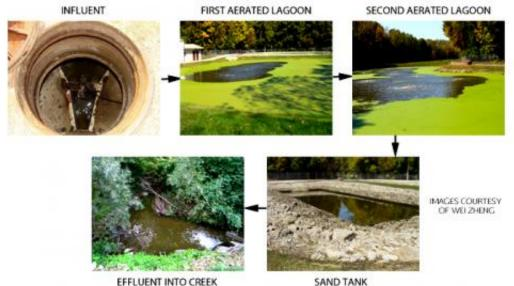
Wastewater, called the influent, is pumped from homes to the sewage treatment facility. This water is then pumped through a series of lagoons, either aerated or not, that contain microorganisms to degrade contaminants like pharmeceuticals, personal care products (PPCPs) and hormones. The water is pumped into a sand tank for further filtration, then the effluent is finally discharged into a creek or other body of water.
