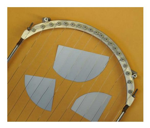
Pieces of a silicon wafer (in gray), used for solar cells or computer chips, can be coated or "passivated" using a vapor deposition process, in which the wires shown here are heated to vaporize polymer materials which then are deposited to coat the surface. Credit: Felice Frankel
