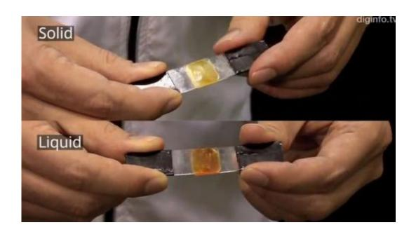
(Phys.org)—Researchers at Japan's National Institute of Advanced Industrial Science and Technology, (AIRT) have developed an organic material that can be liquefied or hardened by shining different types of light on it. The result is an adhesive that can be used over and over again.
