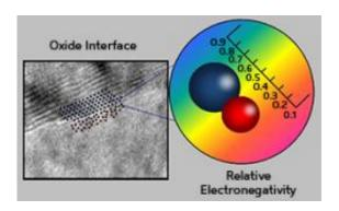
A new theoretical model enables accurate predictions of dipoles at oxide interfaces (left, electron microscopy image) using the classical property of electronegativity (right). The scale shows how two elements with different relative electronegativities align at an interface. Credit: 2013 A\*STAR Institute of Materials Research and Engineering
