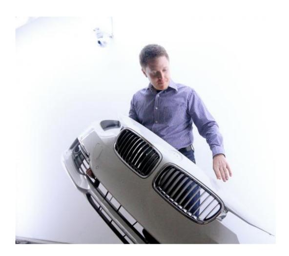
A point of the finger is all it takes to send the defect in the paint to the QS inspection system, store it and document it. Credit: Fraunhofer IOSB
