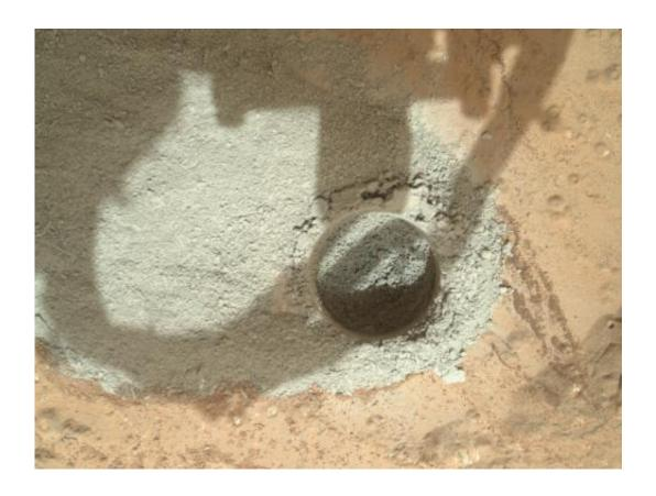
In an activity called the "mini drill test," NASA's Mars rover Curiosity used its drill to generate this ring of powdered rock for inspection in advance of the rover's first full drilling. Credit: NASA/JPL-Caltech/MSSS
