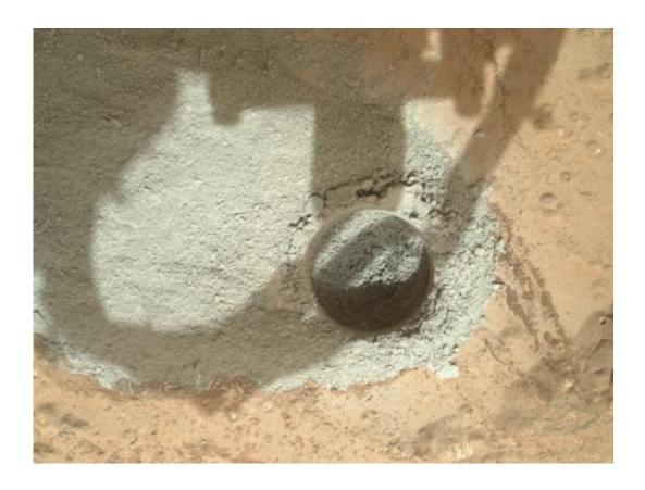
In an activity called the "mini drill test," NASA's Mars rover Curiosity used its drill to generate this ring of powdered rock for inspection in advance of the rover's first full drilling. Credit: NASA/JPL-Caltech/MSSS
