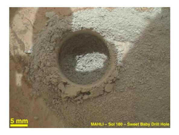
After an activity called the "mini drill test" by NASA's Mars rover Curiosity, the rover's Mars Hand Lens Imager (MAHLI) camera recorded this close-up view of the results during the 180th Martian day, or sol, of the rover's work on Mars (Feb. 6, 2013). Credit: NASA/JPL-Caltech/MSS
