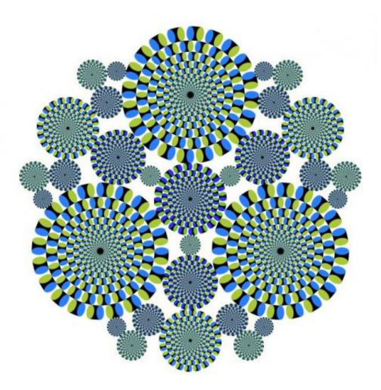
Two-dimensional space- lling bearing con guration with 31 rotor disks. In order to suppress gliding friction, disks rotate either clockwise or anticlockwise, all with the same tangential velocity, and loops of touching disks always have an even number of disks. This static illusory-motion image is an adaptation from
