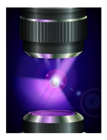
Thanks to this setup, a "cold" laser beam hits a sample at the center; a camera then analyses the phase (holographic technique) and a computer builds a 3-D image of the sample -- including its interior. Credit: Yann Cotte - Fatih Toy - EPFL
