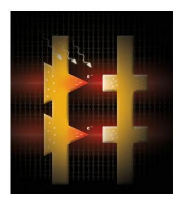
Illustration of a working nanosized optical rectifying antenna or rectenna. Credit: Brian Willis
