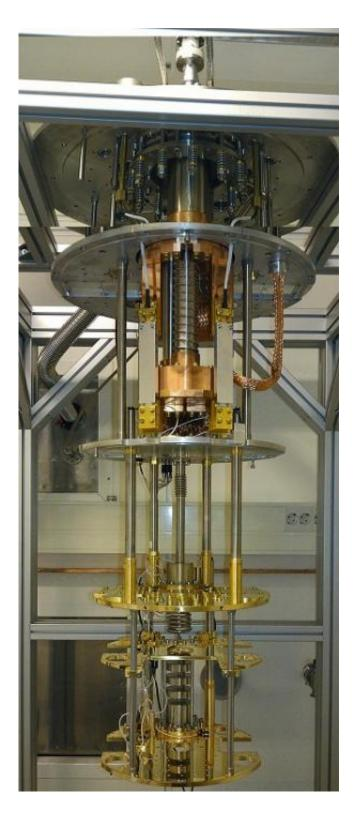
This image shows how the measurements were made. This open dry dilution fridge by BlueFors Cryogenics is similar to the one where the measurements for the study were made. This one is capable of reaching temperatures below 7 mK
