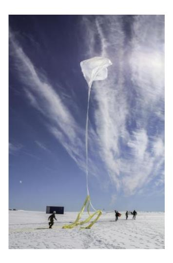
Scientists race through the Antarctic snow to launch one of 20 balloons as part of NASA's BARREL (Balloon Array for Radiation belt Relativistic Electron Losses) mission. Each balloon is equipped with instruments to help track how electrons from giant radiation belts surrounding Earth travel down magnetic field lines toward the poles. Credit: NASA/S. Spain
