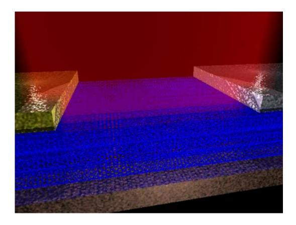
This illustration shows an array of parallel carbon nanotubes 300 micrometers long that are attached to electrodes and display unique qualities as a photodetector, according to researchers at Rice University and Sandia National Laboratories. Credit: Sandia National Laboratories
