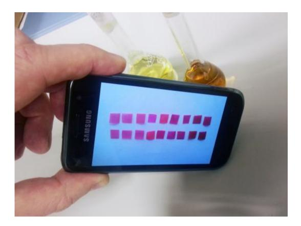
The mobile detects the differences in the color of various membranes submerged in waters with varying mercury concentrations. Credit: J. M. García et al.
