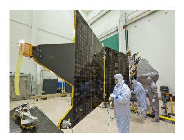
NASA's MAVEN spacecraft recently completed assembly and has started environmental testing. In the Multipurpose Test Facility clean room at Lockheed Martin, technicians installed the orbiter's two solar arrays prior to a modal test. Credit: Lockheed Martin
